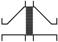
**Bi-directional in-line detonation flame arrester**
